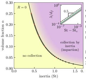
Curve is line of phase transitions, below it no droplets collide with fibres, at it droplets start to collide with fibres
