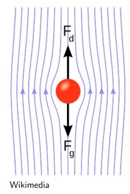
Droplet diameter d falling in air feels two forces: gravity and drag. Falls to ground in
