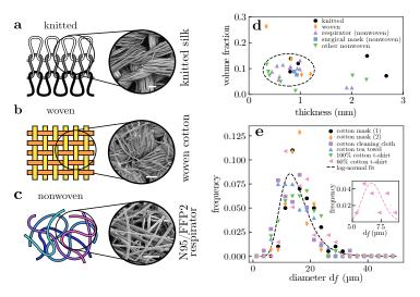
fabrics around 1 mm thick, and about 15 % fibres and so 85 % air. Made of fibres tens of  $\mu m$  thick.
