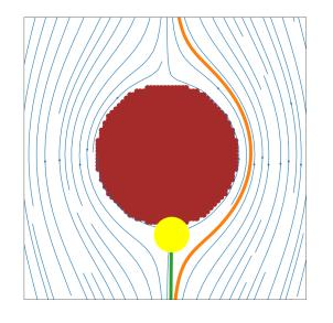
Orange trajectory, drag force dominates inertia, so droplet follows air streamlines (blue) and moves around fibre (red) so is not filtered
