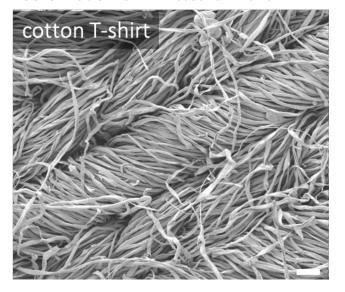
scalebar 100  $\mu m$   $\,$  note structure is basically hierarchical with smallest fibres  $\sim$  10  $\mu m$
