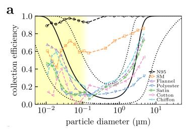
efficiency high for large and small droplets, low for droplets between  $0.1\,\mu m$  to  $1\,\mu m$
